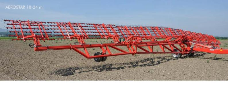
All sections of the semi pull type version of the AEROSTAR are attached to suspend beams. These beams are hydraulically controlled (hydraulic level adjustment).
