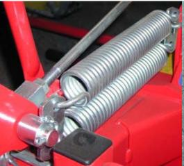
Implements with a working width of 4.5 m and 5 m / 14.8 ft and 16.4 ft fold manually or hydraulically and are spring supported.
