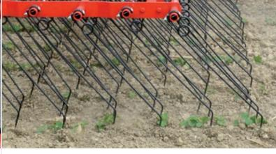
The **hydraulic tine adjustment** will make using the AEROSTAR-EXACT in changing soil conditions a whole lot easier. It also puts the tines in a flat angle when the AEROSTAR is folded.
